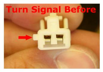
Of course that is because the socket is powering 2 lights - the parking light and the brake light. The plug WILL FIT over either the two left or the two right pins if you grind off the tab:
