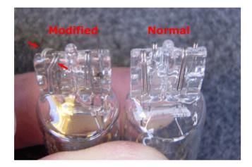
Now the turn signal plug over only two of the pins will power the brake light bulb, which is the same intensity as the turn signal bulb, and your blinker will flash normally. Sure we'll only be using half the bulb, but that's what I came up with for now. There are differences between the single filament turn signal bulb and the dual filament bulbs so you cannot (easily) plug them into the other's socket.
