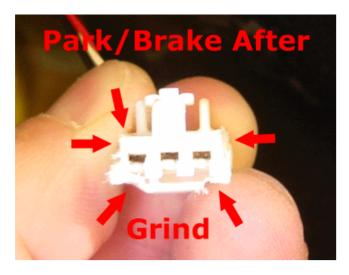
Notice the red arrows pointing to the areas that were ground away. Now this plug will fit into the new 2004 taillight LED park/brake socket! AND the wires are correct, no swapping/cutting/splicing is necessary. You're done with the park/brake light. FYI - in the first pic the right (which is bottom on the light) pin is a Common Ground (-), the middle pin is parking light 12V positive (+) and the left (top) pin is brake light 12V positive (+).
