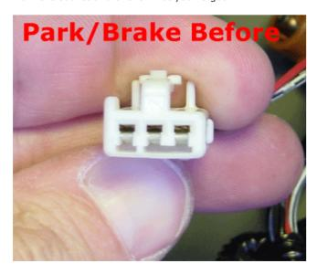
The only difference between these two plugs is the old one doesn't have the notches cut out of it to allow it to plug into the new park/brake led module. Note the red arrows pointing at the tabs in the first picture. I took a dremel tool and notched the plug at the corners and took that big tab off the one side on the top. It's not pretty but this is what we have now:
